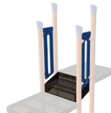
Deck-to-Deck ADA Transition Stair Available for 3.5" and 5" posts 12", 16", 24", and 36" elevation change
